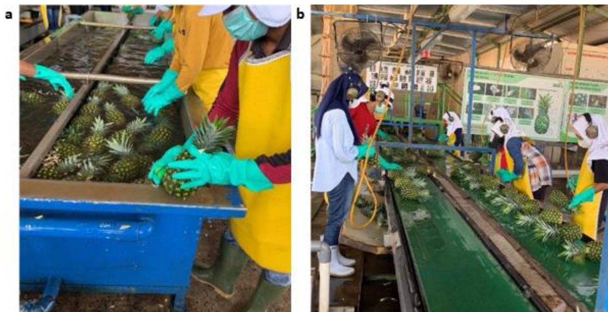
a: Pineapples being brushed and washed in a water tank. b: Pineapples being individually cleaned with HPA.
