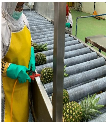
Figure 2.18 Pineapples being treated with fungicide
