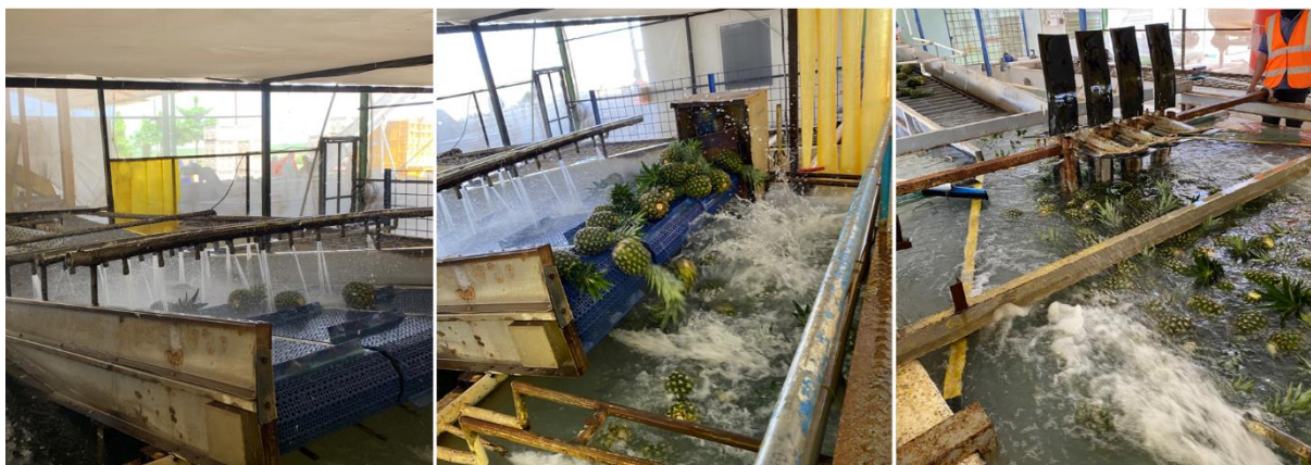
Figure 2.17 Pineapples undergoing second wash with chlorinated water
