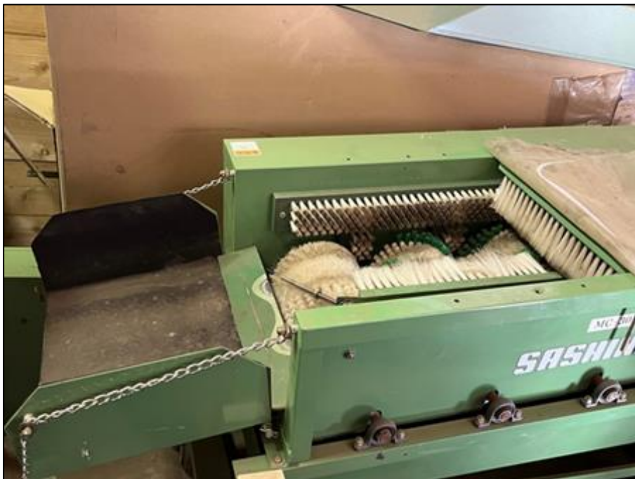
Figure 2.10 Machine for brushing and cleaning melon fruit
