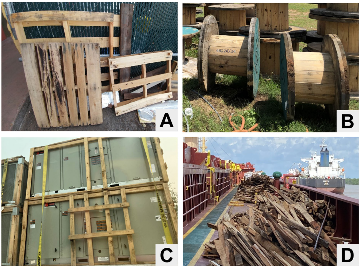
Fig. 1 Wood packaging material (WPM) is the term for solid wood products used to aid in the transportation, protection, or containment of commodities. Wooden pallets (A) are the most common WPM used to facilitate the movement of packaged and bulk goods within warehouses, in trucking, and in shipping containers. Wooden packaging like spools (B), crates (C), cases or frames that contain or protect a commodity are also WPM. Blocks, strapping, and other wooden materials used to
