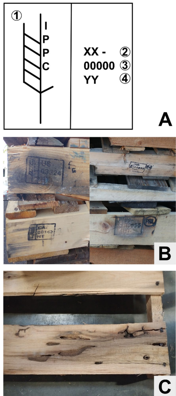
Fig. 5 An example (A) of the mark required under the International Standard for Phytosanitary Measures (ISPM 15); Regulation of Wood Packaging Material in International Trade. Each mark is required to show the International Plant Protection Code (IPPC) logo (1); the country code (2); the facility code where treatment was applied (3) and the type of treatment applied (4); versions of that mark (B) as applied to pallets; and a pallet showing pre-milling insect damage (C). Illustration by CJK MacQuarrie; Photo credits: LF Greenwood
